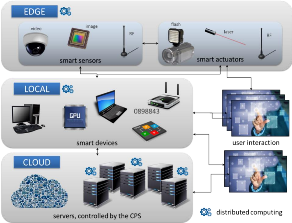
Generic configuration of imaging and video pipelines in CPS.
