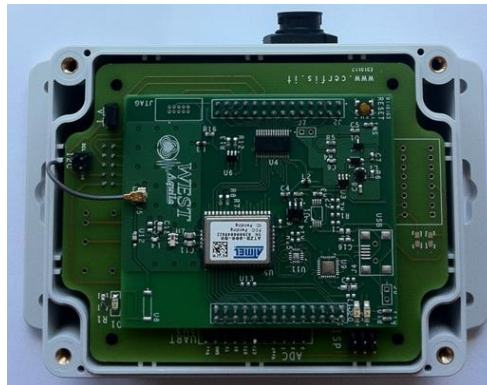
Figure A3.3 - WESTmote sensing platform with IP-65 compliant packaging
